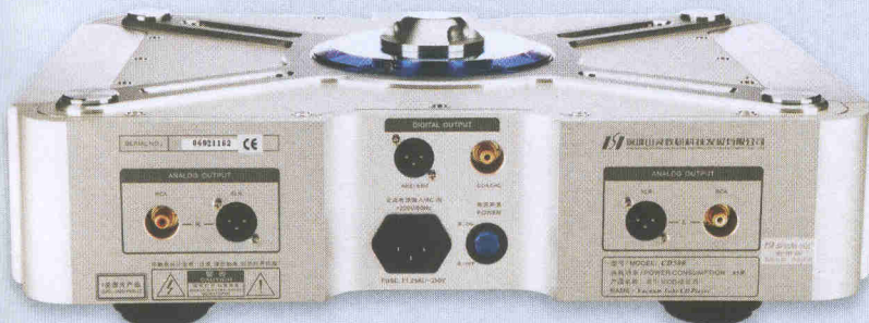
ABOVE: Rear panel includes single-ended and balanced (XLR) analogue outputs plus S/PDIF (phono) and AES/EBU (XLR) digital outputs
